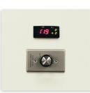
Separate thermostat and fan control on door.
